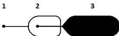
Fig. 1. Design of the microfluidic device: (1 – oil inlet, 2 – aqueous inlet, 3 – reservoir). The width of the channel was 100 \mu\text{m} and the height was 25 \mu\text{m} .
