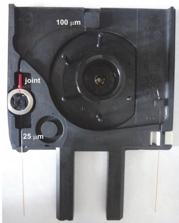
Fig. 1 Photograph of a coupled capillary inserted into a cassette.
