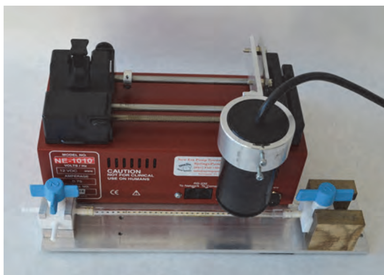
Fig. 1. Photograph of the device for DLTV with a tubular chamber and a syringe pump for diode laser advancement. A preprinted paper strip is inserted in the chamber.
