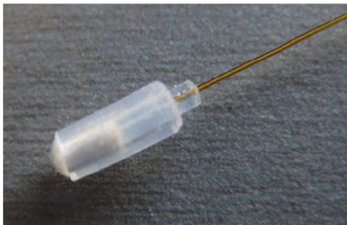
Fig. 1: Connection of the filtration cartridge to the anodic end of the fused-silica separation capillary.
