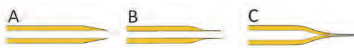
Fig. 2: Profile of electro spray tips. A – grind tip, B – etched tip, C – pulled tip
