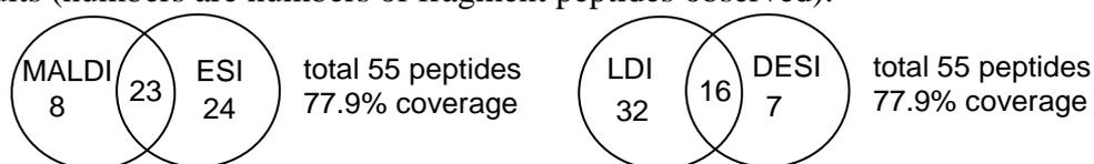
The LDI/ DESI combination gives peptide coverage comparable to MALDI/ESI, but with the added advantage of a common sample format, thereby enabling deeper analysis of a sample spot that would otherwise be only amenable to MALDI analysis.
