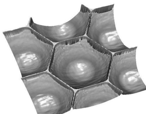
Additional software and exposure strategies have been implemented into the laser lithography systems to alleviate the design process and increase the quality of the exposed structures. There are several methods to increase the surface quality at the cost of write speed. With full optimization a surface roughness below 10nm was achieved.
