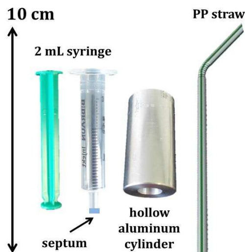
Figure 1. The photo of the consumables used to build a miniature EBC sampling device.
