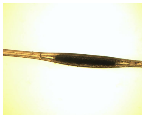
Fig. 1. Microscopic view of the paper strip laminated in the pouch
