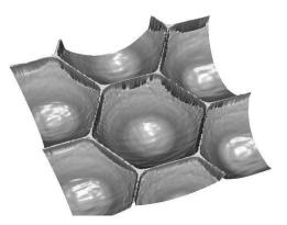
standard positive photoresists but also on the negative photoresist SU8 that offers good chemical, mechanical and optical properties for different applications [2,3]. Because SU8 is a negative photoresist the exposures had to be made from the backside of the substrate, exposing through the glass.
