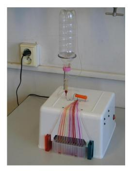
The solution of current compromises of CF IEF is seen in combination of the features of small separation channels with those of large ones. The basic idea comprises the continuous widening of the flat channel while the liquid flows from channel input toward the outputs which generates a divergent flow and, at the same time, the use small voltage at the channel input and high voltage at the channel output.
